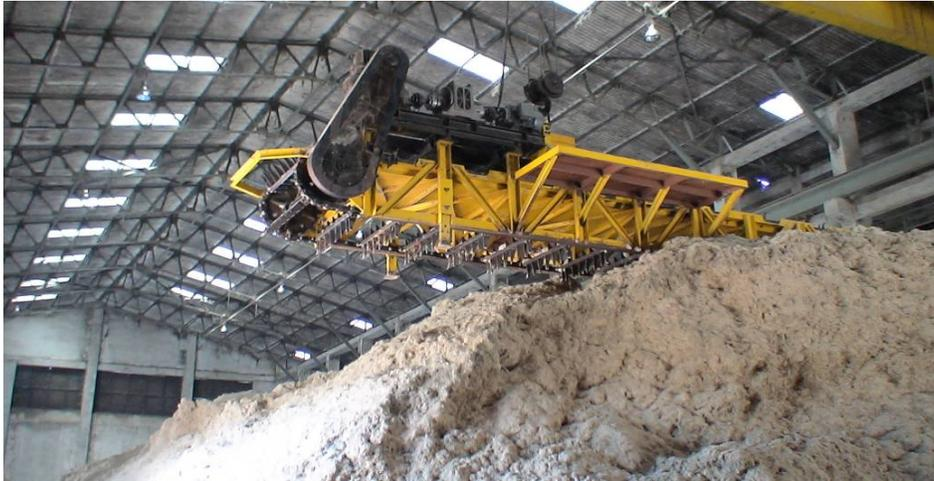
**CLOSED STORAGE BAGASSE STACKING AND RECLAIMING SYSTEM**
